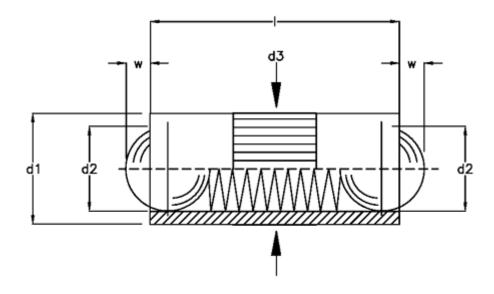
$\begin{array}{lll} d1 & = 4.0 \\ d2 & = 3.0 \\ d3 & = 4.03 \\ I & = 9.0 \\ Spring \ pressure \ N \ bottom = 7.5 \\ Spring \ pressure \ N \ top & = 2.5 \\ W & = 0.90 \\ \end{array}$
